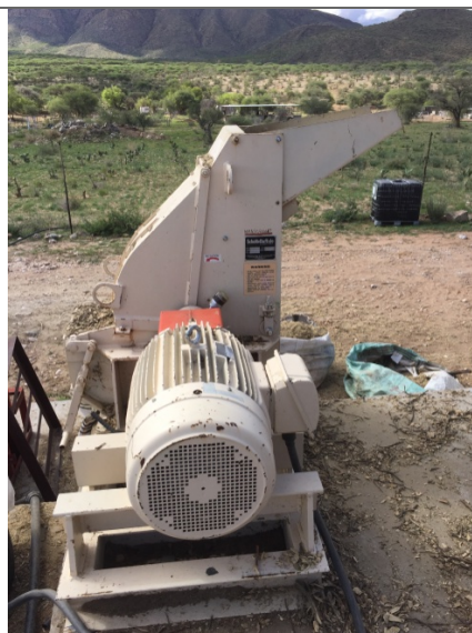
Picture 11: Buffalo stationary hammer mill installed at Farm Langbeen. The hammer mill is driven by 3-phase electricity and has a throughput capacity of at 0.5t/hr. Due to its size, it is more power and capacity efficient than e.g. tractor-driven types of hammer mills.
