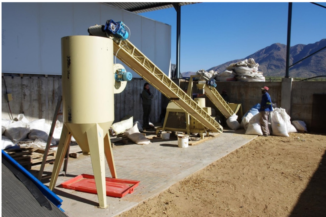
Picture 4: Complete “Jones” pelleting set-up – pellet cooling tower; pellet conveyor; pelleting press; loose feed conveyor; feed mixing bin. (Photo: J. Laufs, Support to De-bushing Project)
