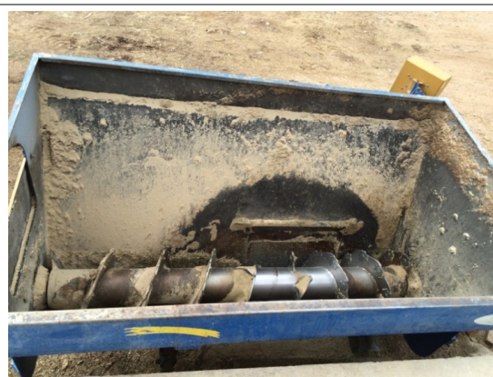
Picture 17: Mixing experimental diets, with a special (large scale), self-propelled feed mixer. This mixer has a capacity of \pm 6\text{m}^3 mixing volume, approximately 400 kg per feed/ diet to be mixed.
