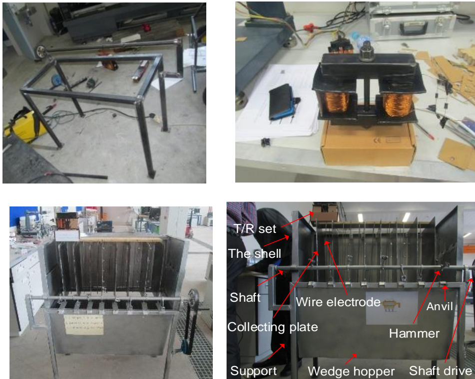
Figure 19: Construction of a mock-up ESP.
