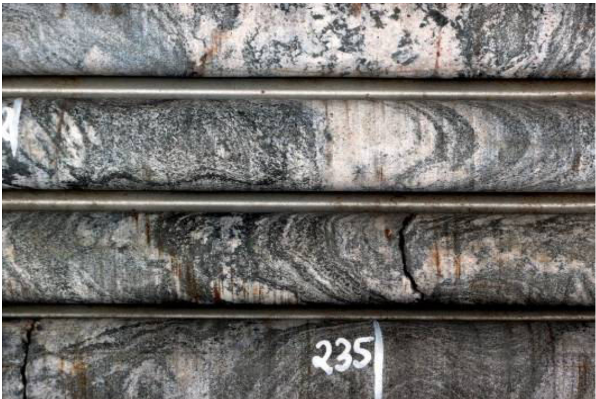
Figure 5.9 Fine medium grained dark grey magnetite bands in folded gneiss at 235 m depth (M63).
