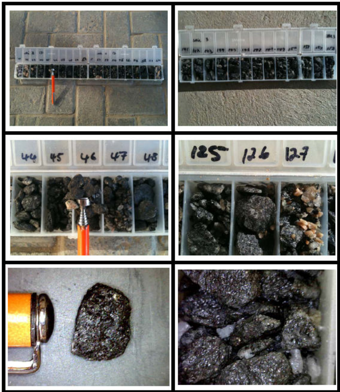
Figure 3.3 Reverse circulation drill chips from hole SHIR3 showing zones of massive magnetite.
