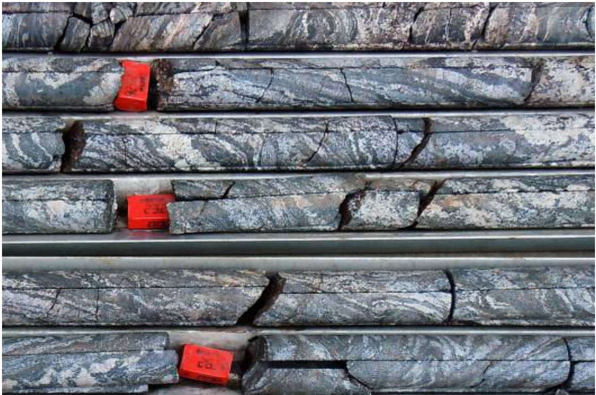
Figure 5.8 Medium to coarse grained dark grey magnetite bands at 23 m depth (M63).
