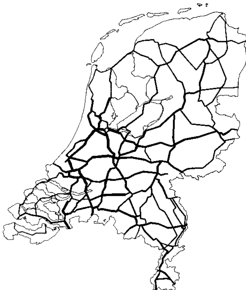
Figure 4. Pattern of main roads in The Netherlands in 1986. The traffic density varies from 10 000 to > 100 000 vehicles per day. The thickness of the lines reflects the area that has a noise load of > 50 dB(A). Source: Anonymous (1991).
