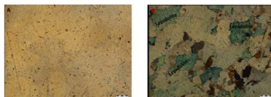
Figure 1. Lepidolite zone under A) PPL and B) XPL.
