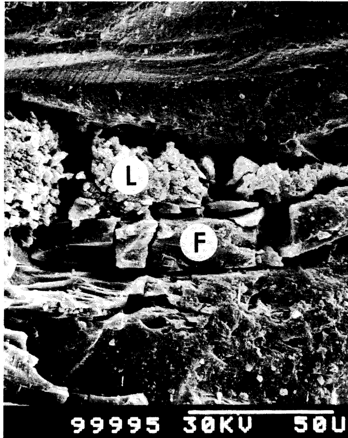
Figure 4: Fragments of quartz (F) in a crack due to mechanical forces exerted by the colonizing lichen. L = areole of colonizing chasmoendolithic lichen.
