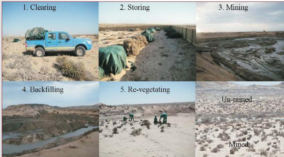
Figure 7. Integration of rehabilitation into mine planning is evident at the Bogenfels mining sites
