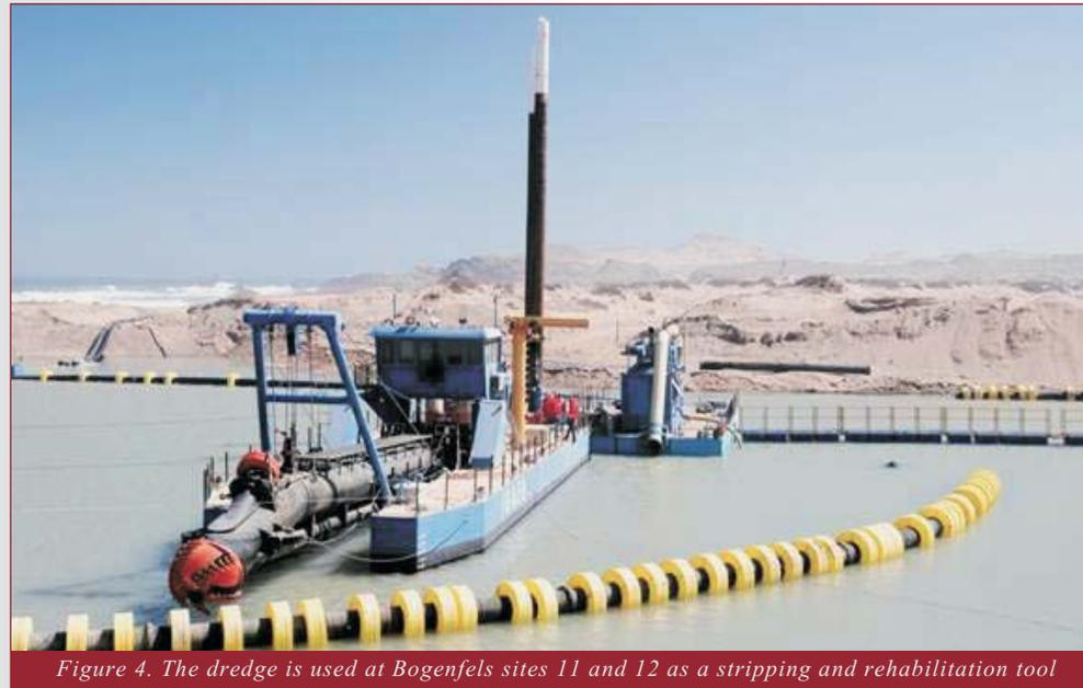
Figure 4. The dredge is used at Bogenfels sites 11 and 12 as a stripping and rehabilitation tool
