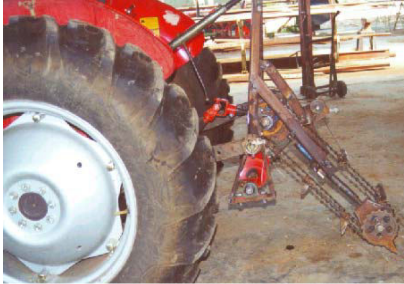
Figure 4h. Tractor mounted trench digger.
