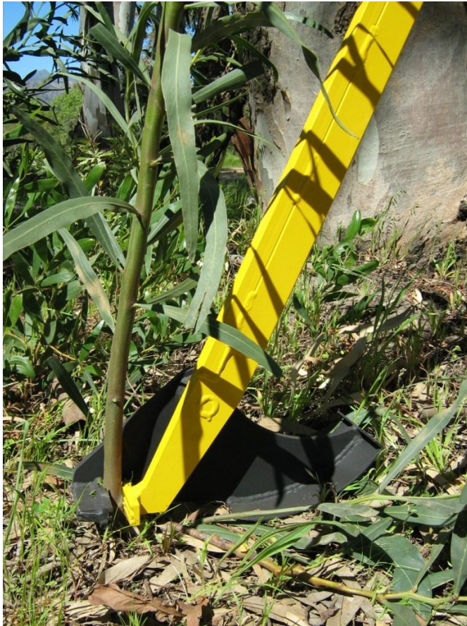
Fig 1: The Tree Popper in action, pulling out an invasive Acacia from Australia in South Africa. (photo from T. Negis).
