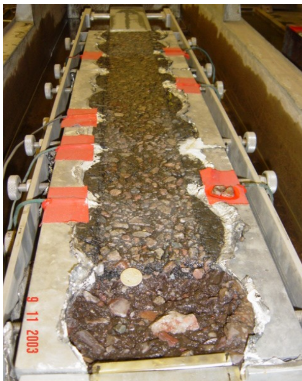
Figure 2. View of test bed showing specimens and clamps in the water tank.
