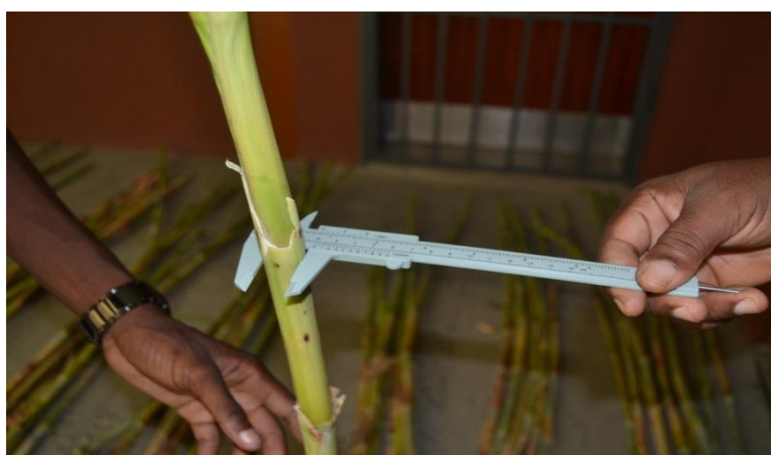
Figure 6: Using Vernier caliper to determine the circumference of the stem of sweet sorghum.
