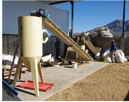
Full view of the Jones pelletiser tested at Farm Langbeem
