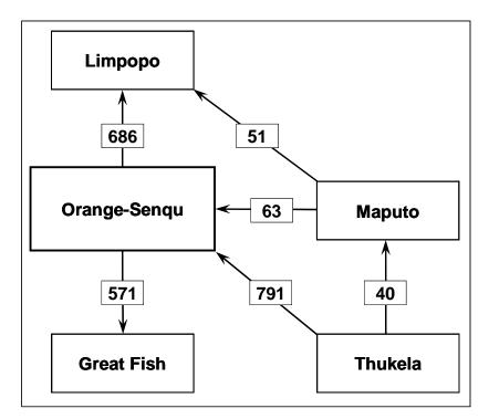
**Figure 2**. Inter-basin water transfers affecting the Orange-Senqu basin. (All water transfers are given in Mm<sup>3</sup>/year; data adapted from DWAF (2003a-e)).
