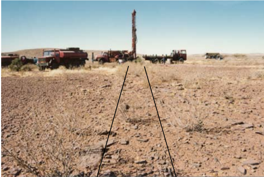
Figure 10: Drill site WW34684, placed on joint in sandstone-shale intercalated Stockdale Formation; RWL expected at >70 mbgl); note up-turned sandstone fragments in foreground, creating an impression of an anticlinal structure.
