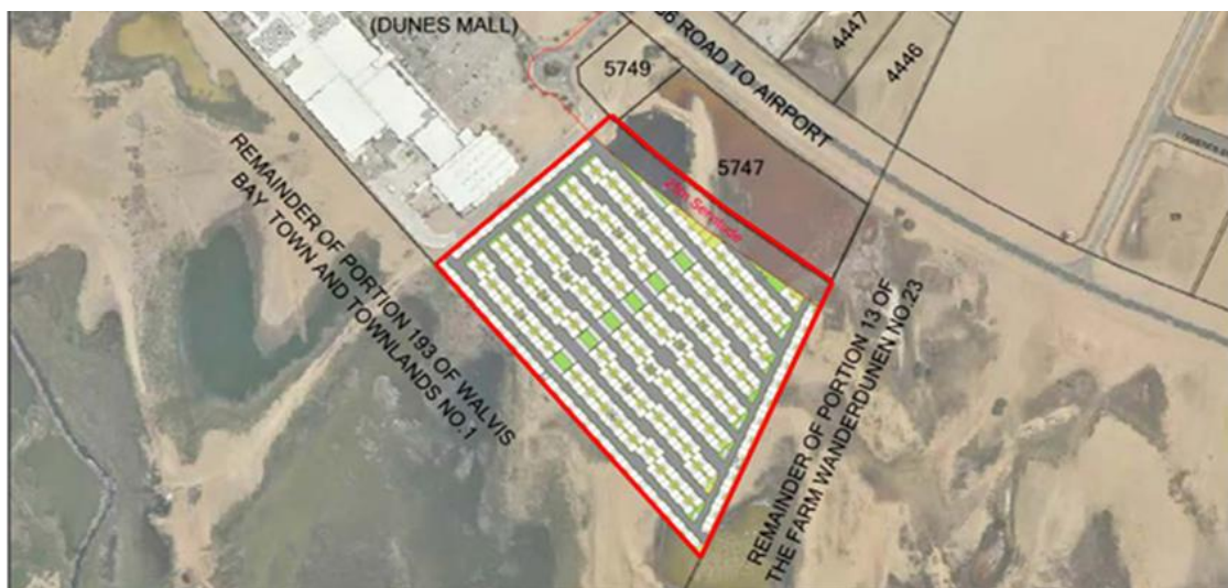
Figure 1: The north-eastern portion of Erf 5748 Walvis Bay contains a 25-metre-wide right-of-way servitude which was taken into account as part of the concept design.
