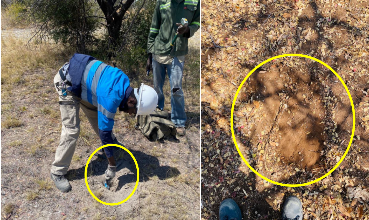
Figure 8. A 30cm soil pit before and after it is backfilled
