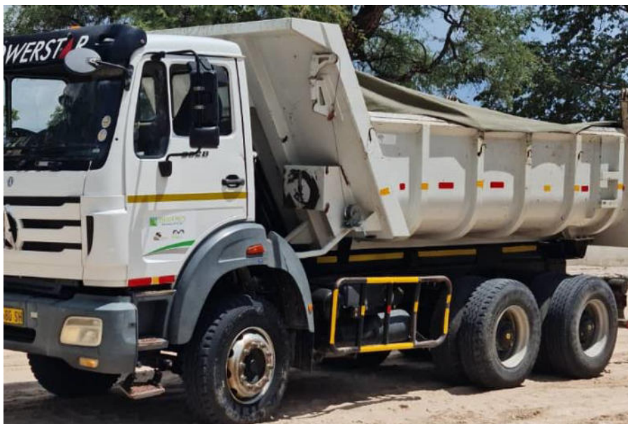
Image 2: Tipper truck used for transportation covered with canvas for dust control.
