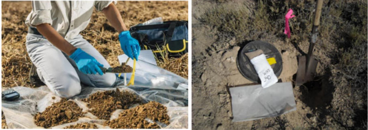
Figure 2-2: Examples of geochemical sampling of soils.
