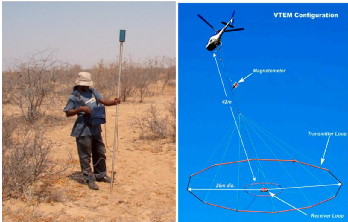
Figure 2-1: A demonstration of the two types of geophysical methods with ground-based magnetometer (left) and airborne magnetometer (right).
