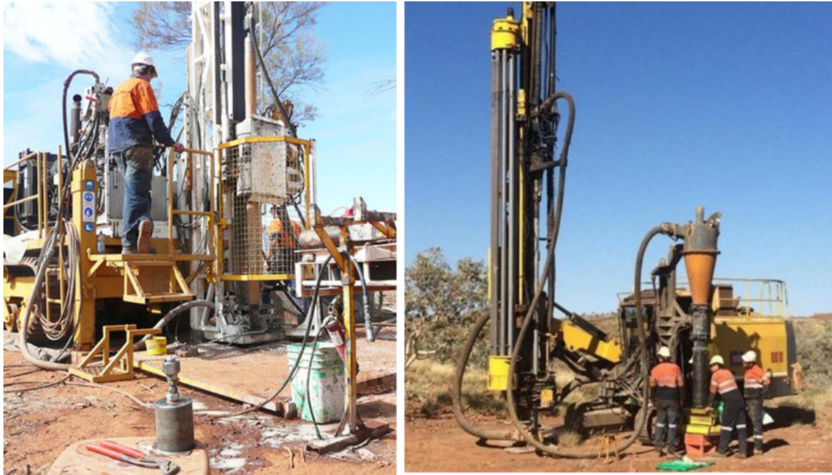
Figure 2-3: Left – diamond drilling and right photo – RC drilling method.
