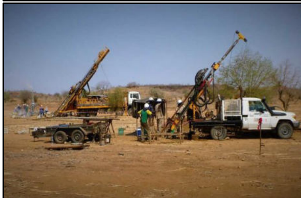
Fig. 13. RC and diamond drilling rigs at work also shown is drill core (activities are very localized with limited footprint).
