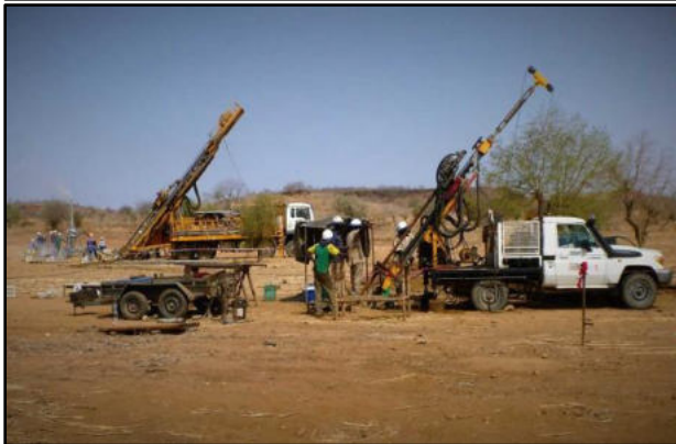
Fig. 14. RC and diamond drilling rigs at work also shown is drill core (activities are very localized with limited footprint).
