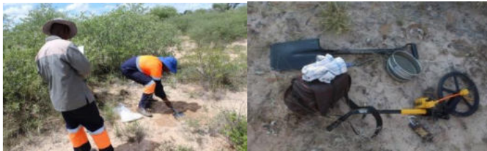
Figure 2-3: An example of soil sample collection and equipment (Resilient Environmental Solutions, 2019)
