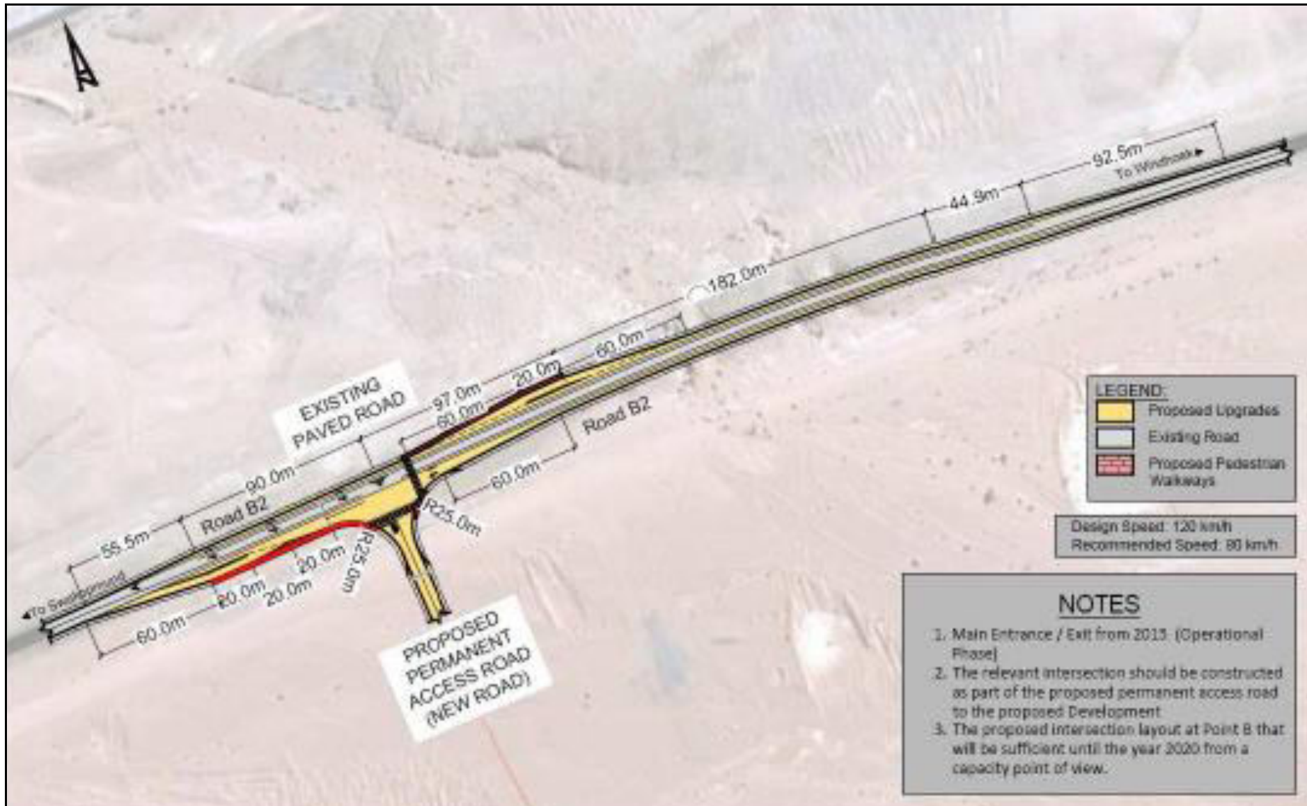
Figure 7-4: Recommended Upgrading of the Intersection of the B2 and the Permanent Access Road (Siyazi, 2010)
