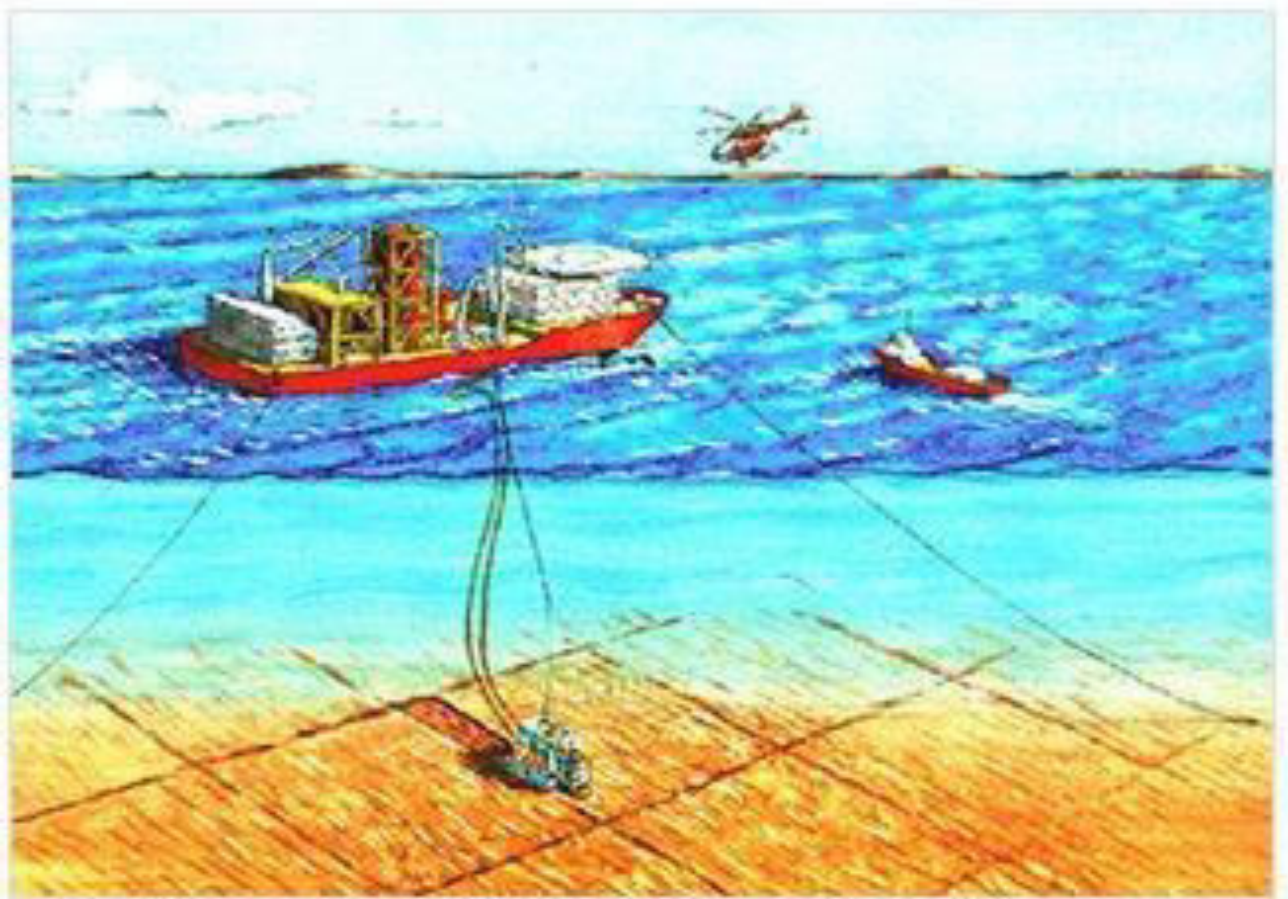
Figure 5: Depict the airlift drilling technology to be used for diamond exploration on the seabed at EPL 5867.
