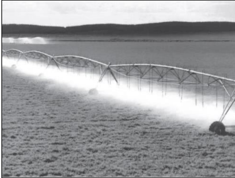
Figure 2-2: The Centre Pivot system overview (Phocaides, 2007)
