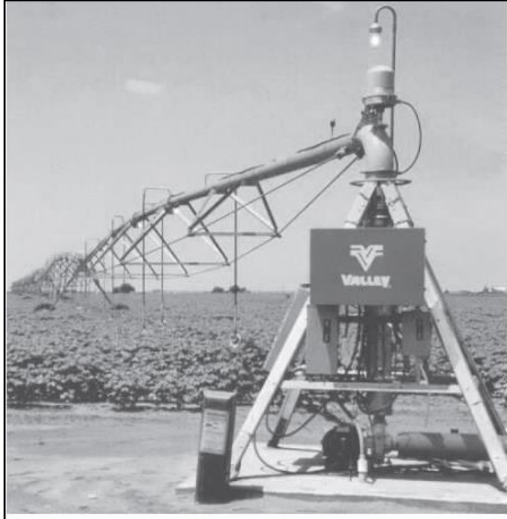
Figure 2-1: The Centre Pivot (Sprinkler) system (Phocaides, 2007)
