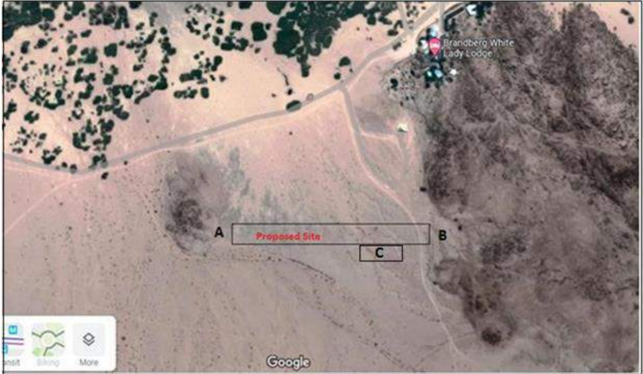
Figure 5: The proposed site marked with letter A and B each indicating where aircrafts will land/take-off (A) and stop (B). The area marked C, is reserved for a building which will be used to provide basic facilities. Tourists will be transported by vehicle to and from the lodge.
