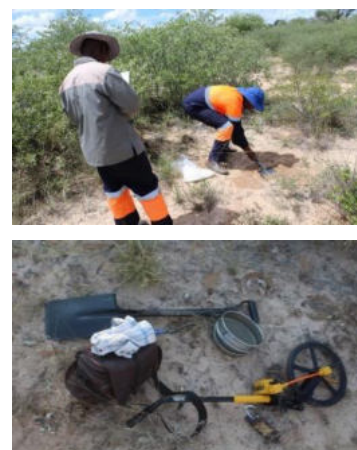
Figure 2-3: Soil sample collection and equipment
