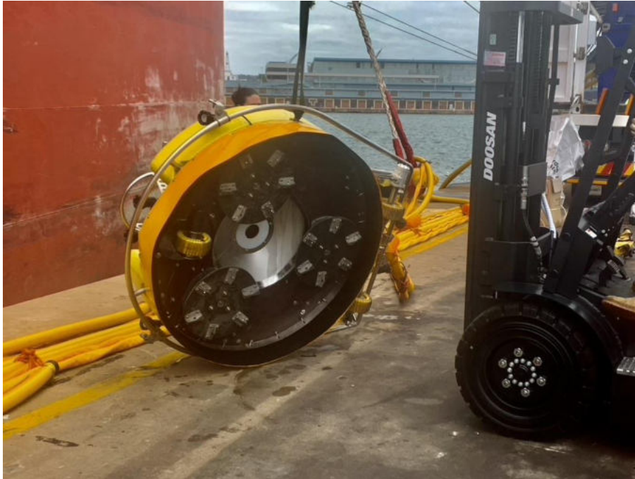
Figure 3: Different cleaning discs and wheels could be fitted to the cart for different cleaning tasks (Schomberg Investments).
