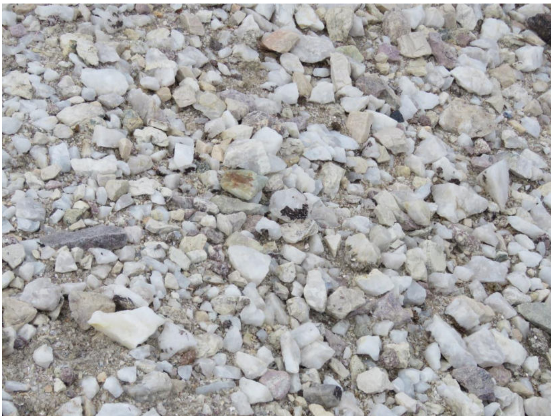
Figure 8: Old tailings on site showing rock fragments of beryl, quartz, feldspar and lepidolite.
