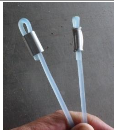
Photo 23. New and more reliable crimping method of attaching baskets to long lines
