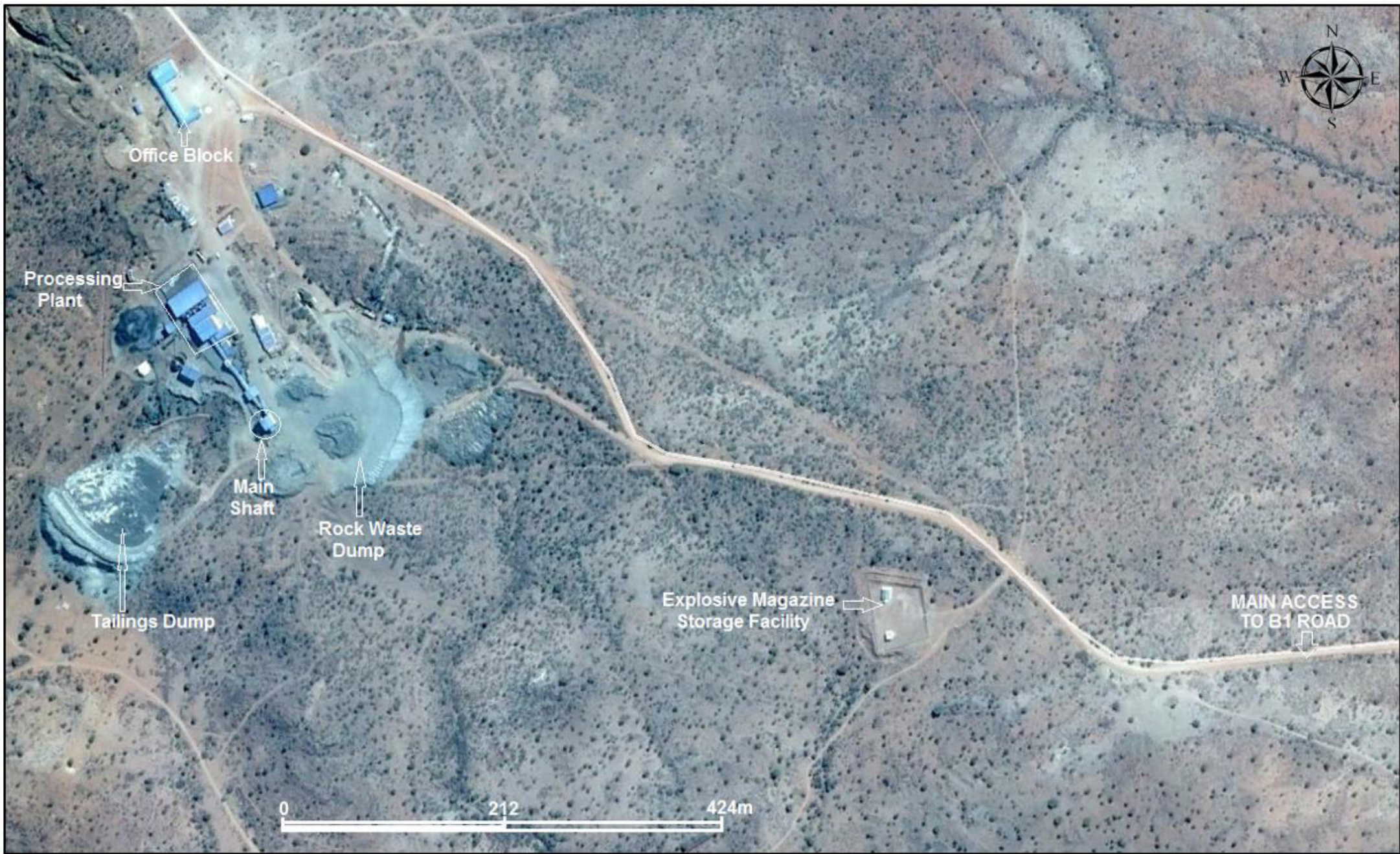
Figure 1.6: Satellite image showing the detailed layout of the Swartmodder Copper Mine in the ML No. 168 (Source: Google Earth, 2022).
