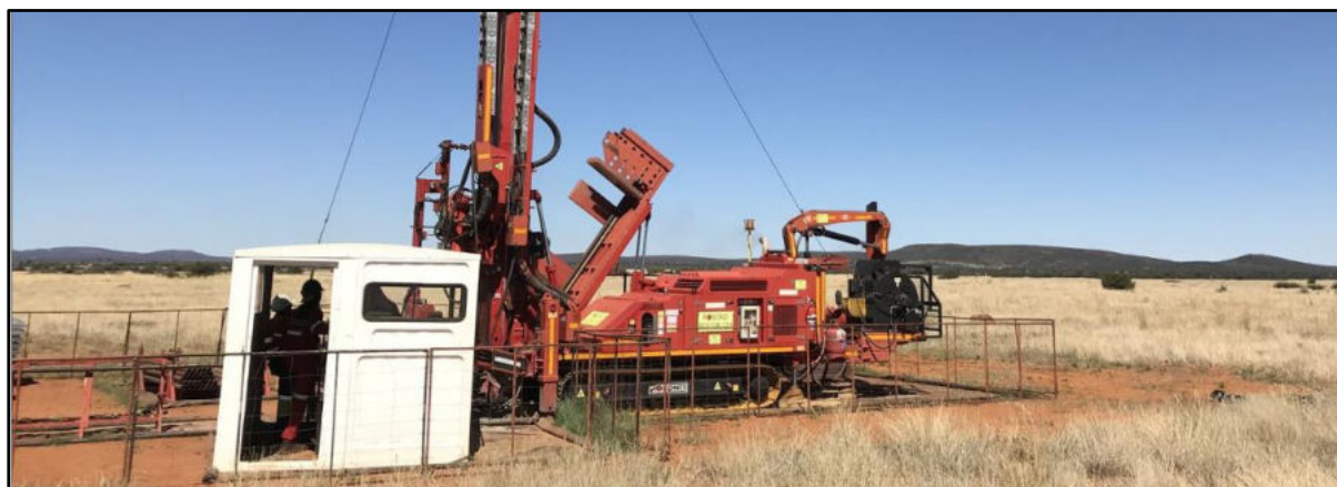
Figure 2-1: A typical example of a Down-The-Hole drill rig.
