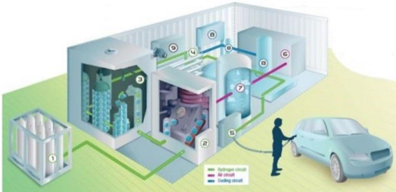
Figure 1-13: Conceptual layout of a hydrogen refuelling station
