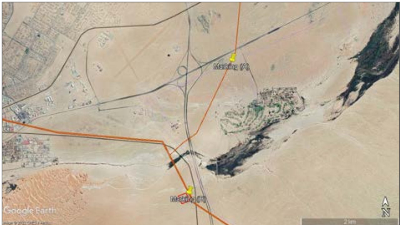
Figure 5-3: Sections of the proposed 66 kV power line recommended for the fitting of marking devices (Marking A to Marking B, 3.3 km), as a mitigation for bird collisions
