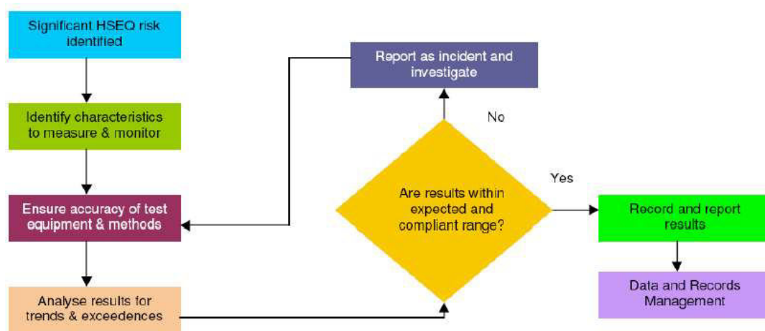
Figure 5.5: HSE monitoring work flow
