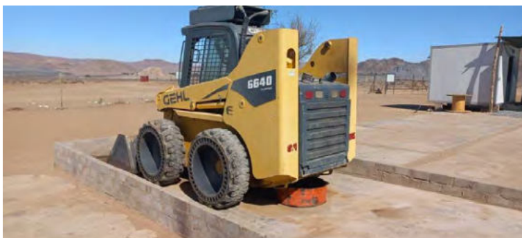
Photo 13 – View of excavator parked within wash bay area and with drip tray. No spillage of oil/diesel was found on either the Contractor's Site office or the construction site.
