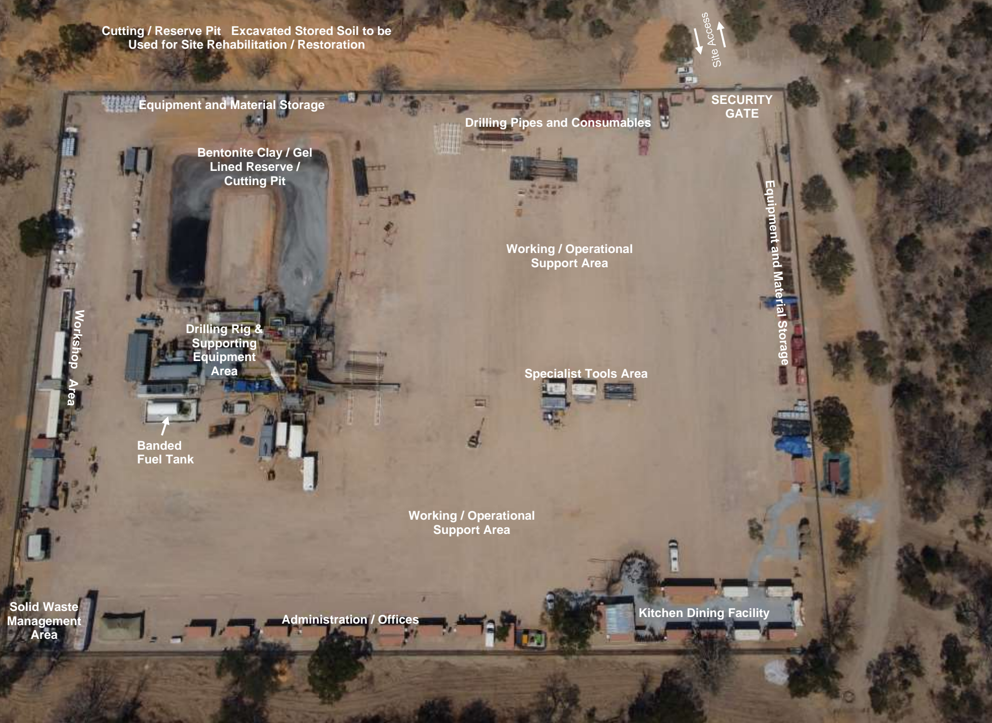
Figure 2.4: Example of an oil and gas well site layout showing a drone view of the 8-2 Makandina well site in Kavango East Region.
