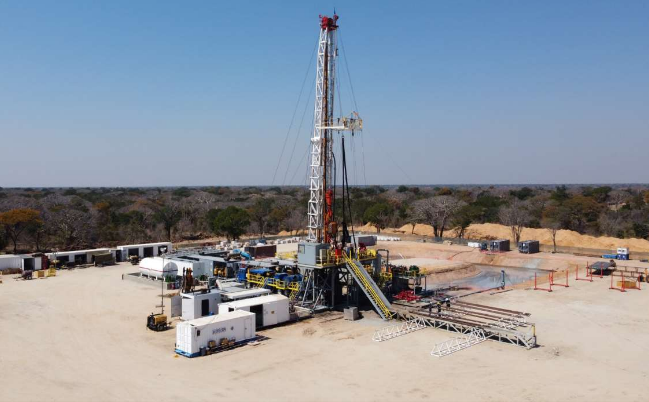
Plate 2.1: The Crown 750 truck mounted drill rig used by REN to drill the stratigraphic wells and will be used to drill the proposed D1-D6 and G1-G6 exploration and appraisal wells in the AOI in PEL No. 73.
