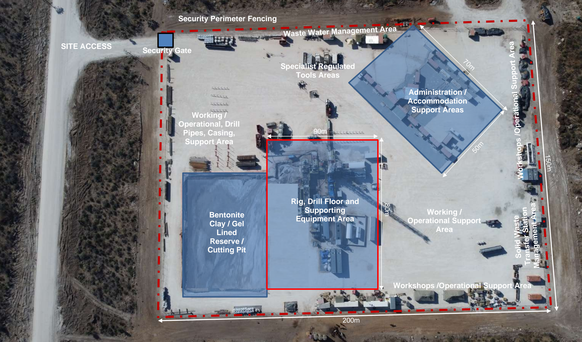
Figure 2.3: Layout example of a typical 3Ha footprint created by an onshore drilling well site coverage superimposed on an actual drilling location and as adopted for the drilling of multiple exploration and appraisal wells within the AOI in PEL No. 73 (Drawn not to scale).
