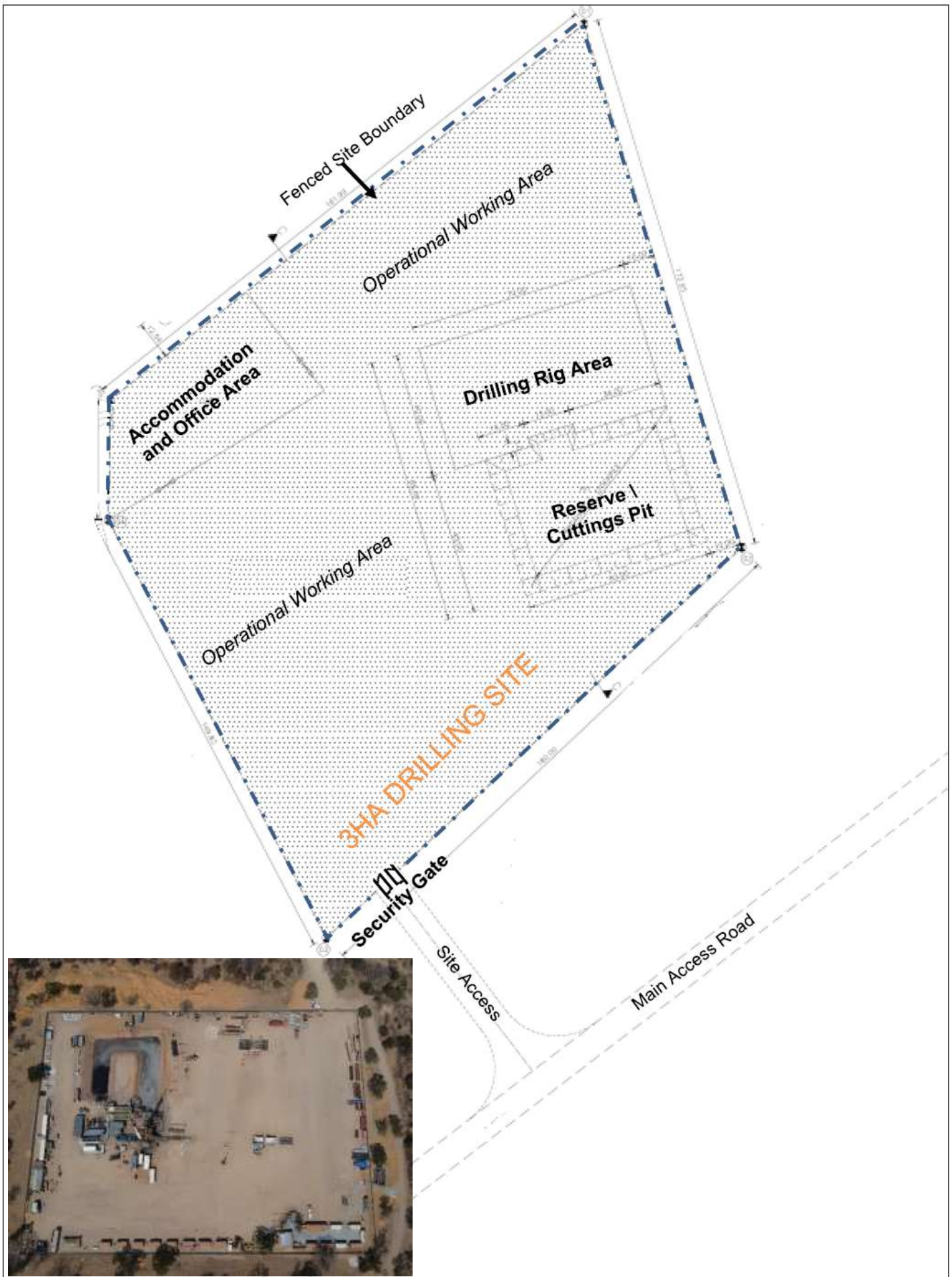
Figure 2.2: Example of a typical 3Ha footprint site coverage showing a general drilling site layout adopted for the drilling of multiple exploration and appraisal wells within the AOI in PEL No. 73.
