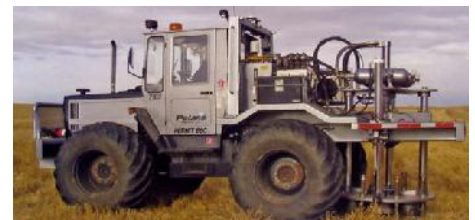
One Explorer replaces 4 larger Seismic trucks. It operates at a low frequency that does not affect wildlife.
