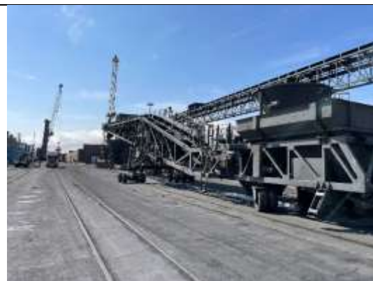
Photo 4-6 Mobile conveyer unit with hopper that is used for initial loading from the vessel.
