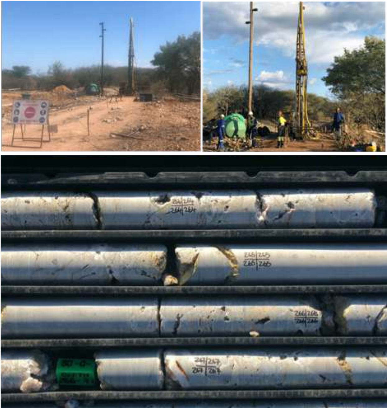
Figure 6. Diamond Core Drilling and Core samples (Safety signs were observed)
