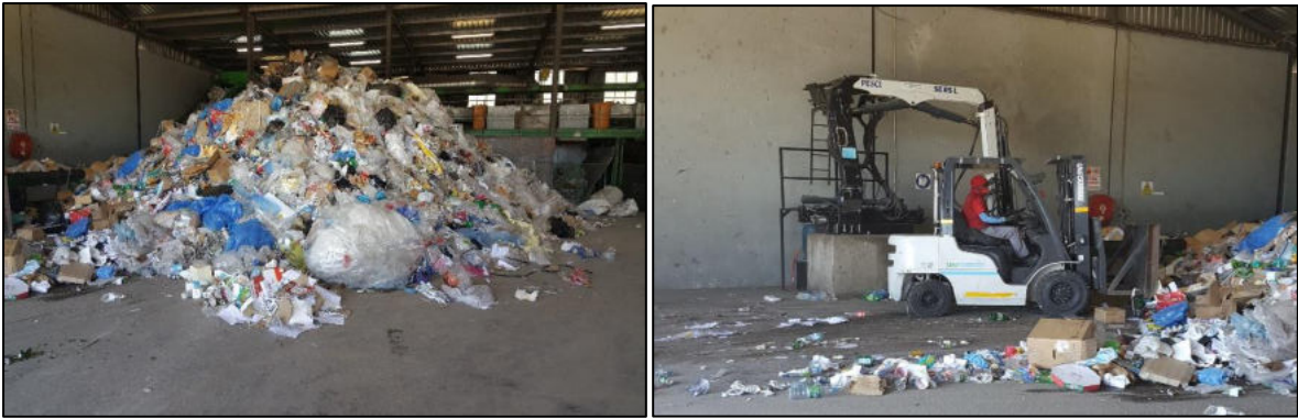
Figure 8: Waste is combined and lifted onto conveyor belt
