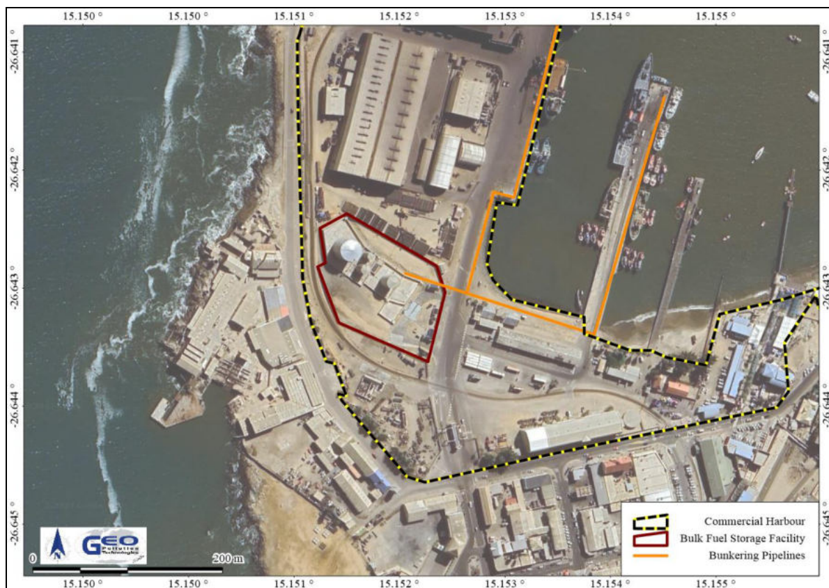
Figure 4-2 Bulk fuel storage facility and pipeline routes
