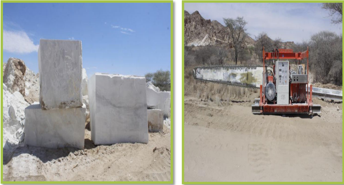
Figure 3: The block of white marble that will be mined and diamond wire saw machine for cutting marble
