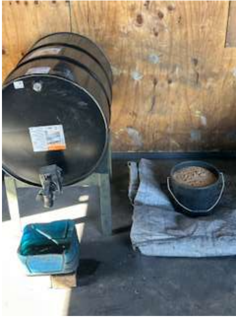
Figure 9 - Presence of a bucket of sand near an oil container to create a temporary bund to contain a spill should one occur.
