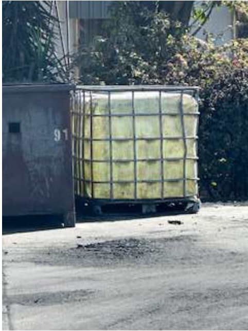
Figure 5 - Depicts chemical tanks situated on an elevated structure that lacks proper bunding (provided by the Proponent)
