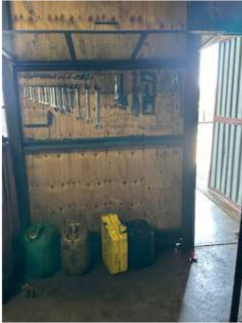
Figure 3 - Fuels can be seen being stored in a dedicated area on a concrete floor (impermeable surface) (provided by the Proponent)
