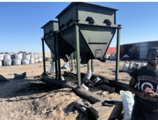
Figure 4: A mobile screening facility is on site to grade the charcoal and ready for packaging
