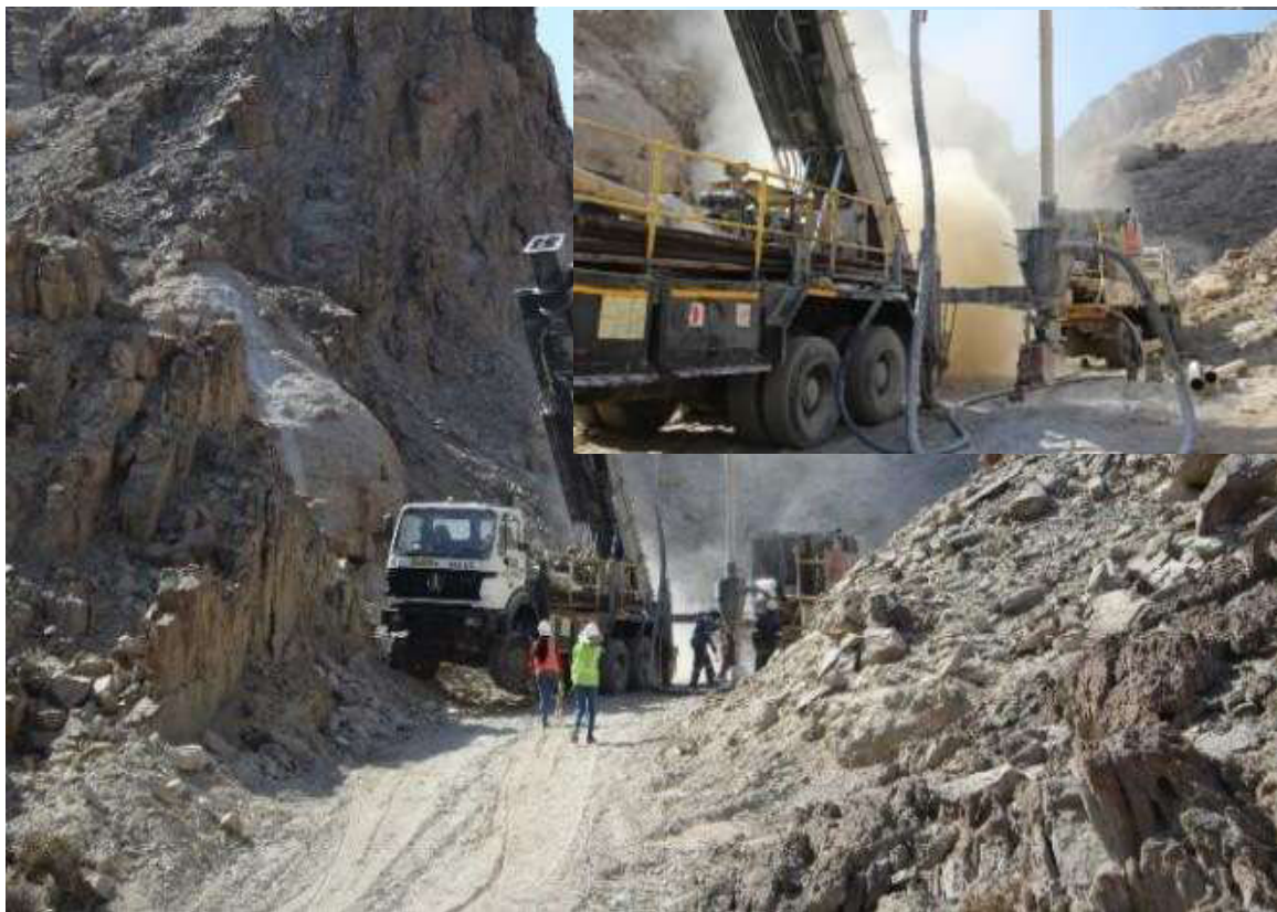
Photo 2, Reverse circulation (RC) drilling equipment at Khan Mine.
