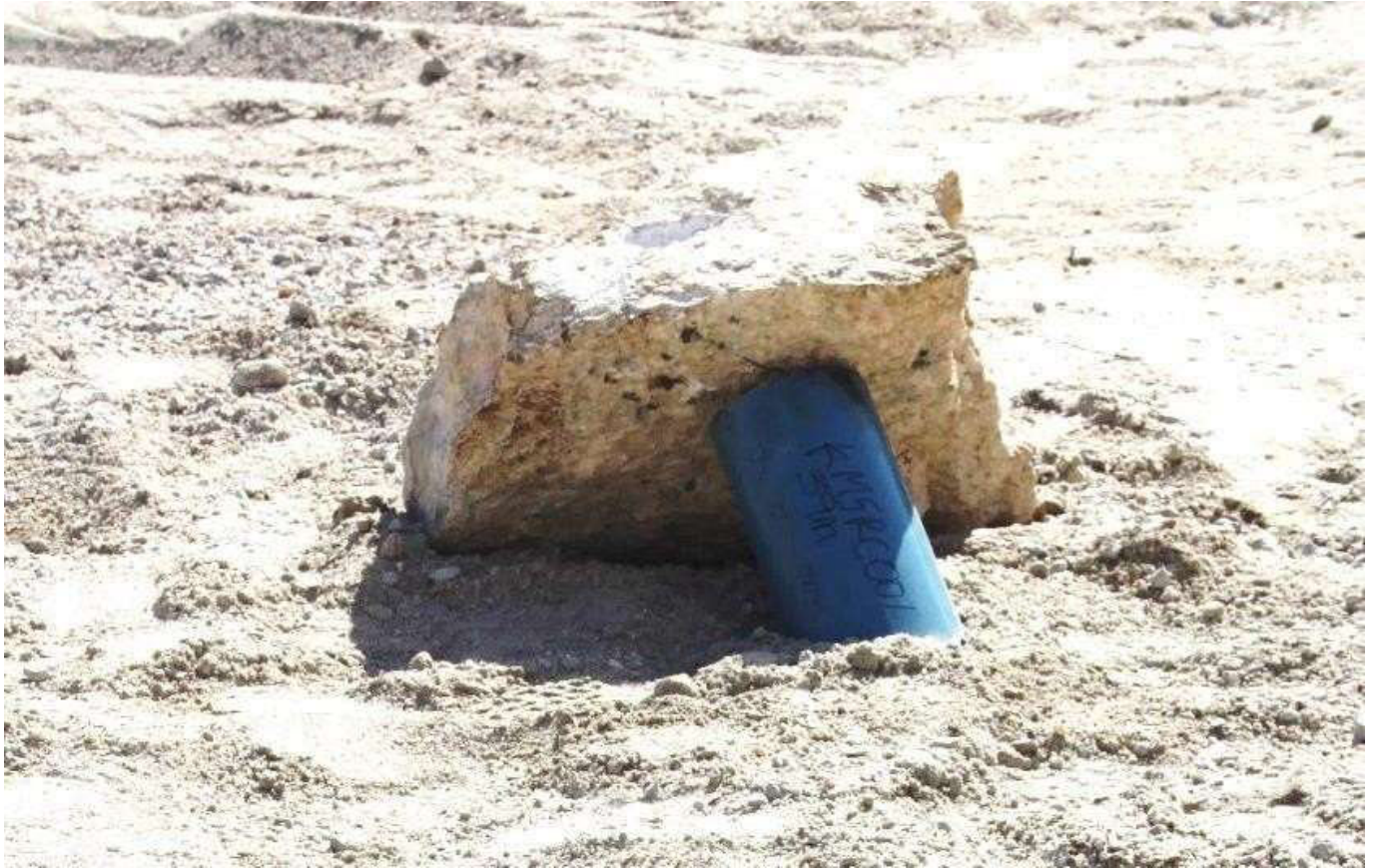
Photo 2 , Drill hole marked and geo referenced, the hole is secured and environmentally safe.
