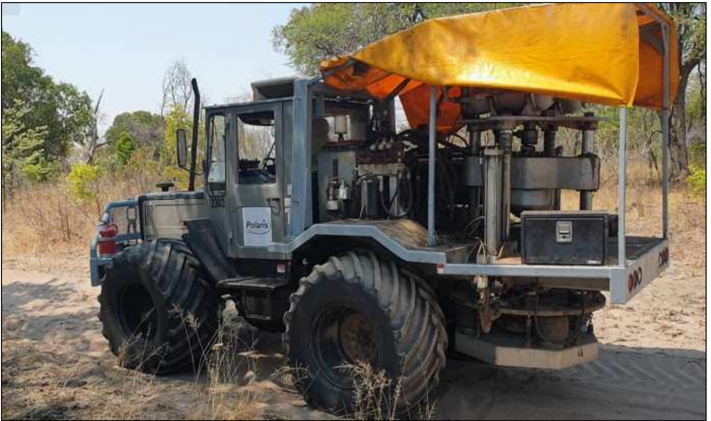
Plate 2.1: The Explorer 860 was used as the energy source for the previous multiple seismic survey operations undertaken in PEL 73.
