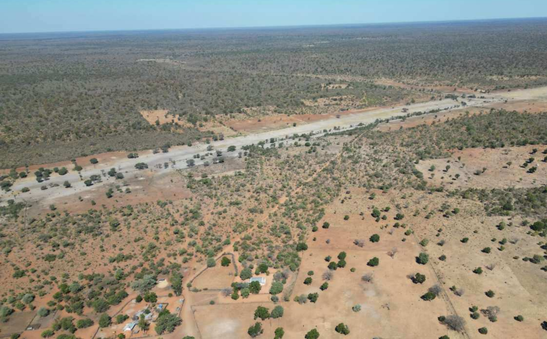
Plate 1.5: June 2024 drone image from Kawe to the south-southwest showing the proposed 2024 Vibroseis test line No. 22-05 (previous Explorer 860 surveyed line) to be undertaken along the existing access and across the Omatako Ephemeral River Channel.
