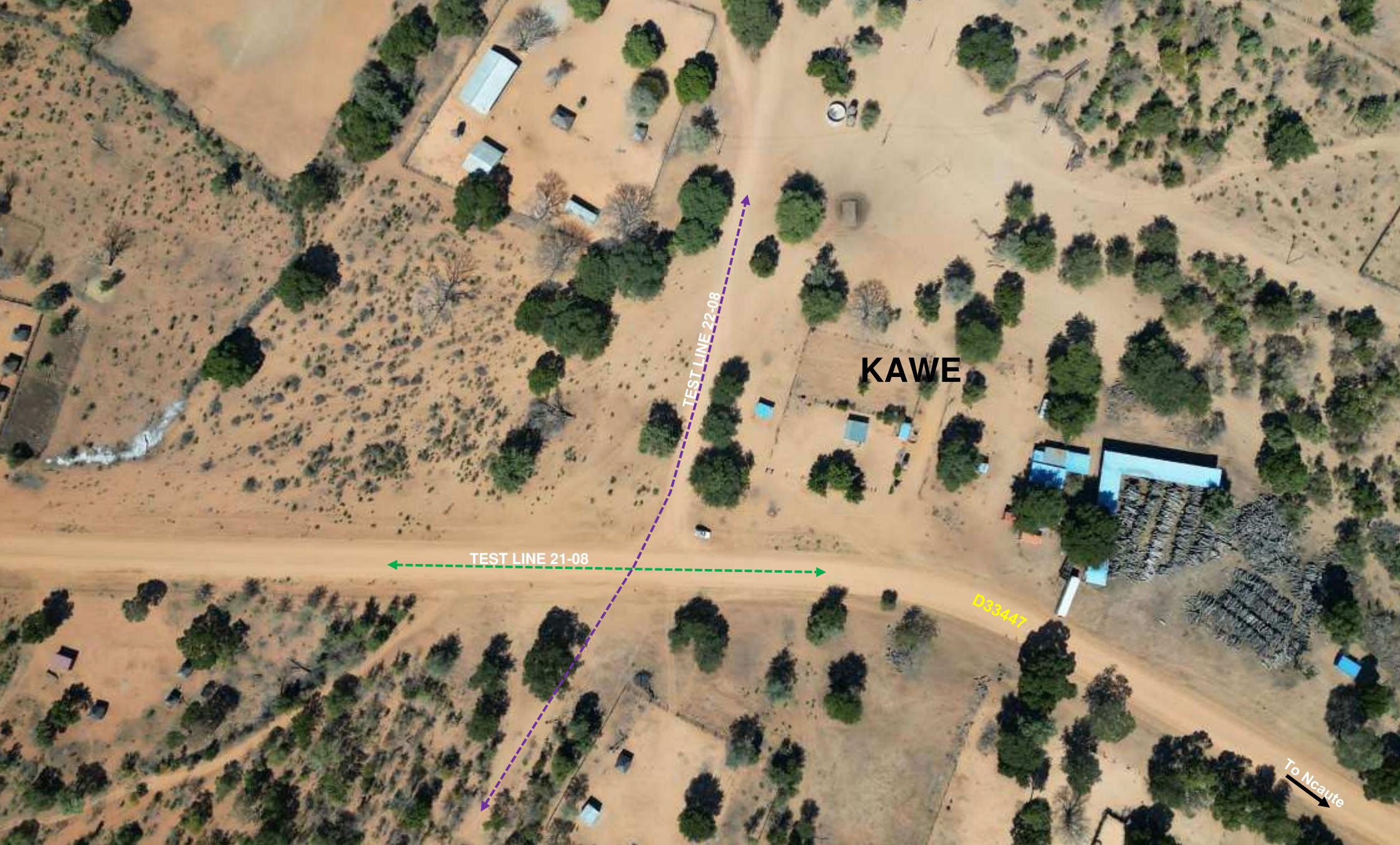
Plate 1.3: June 2024 drone image taken at Kawe where the proposed 2024 Vibroseis test lines 21-08 and 22-05 (previous Explorer 860 surveyed lines) meet. Although Kawe area is congested, the operations can be mitigated by adopting appropriated reduced-force sweeps and application of the appropriate minimum safety distances.
