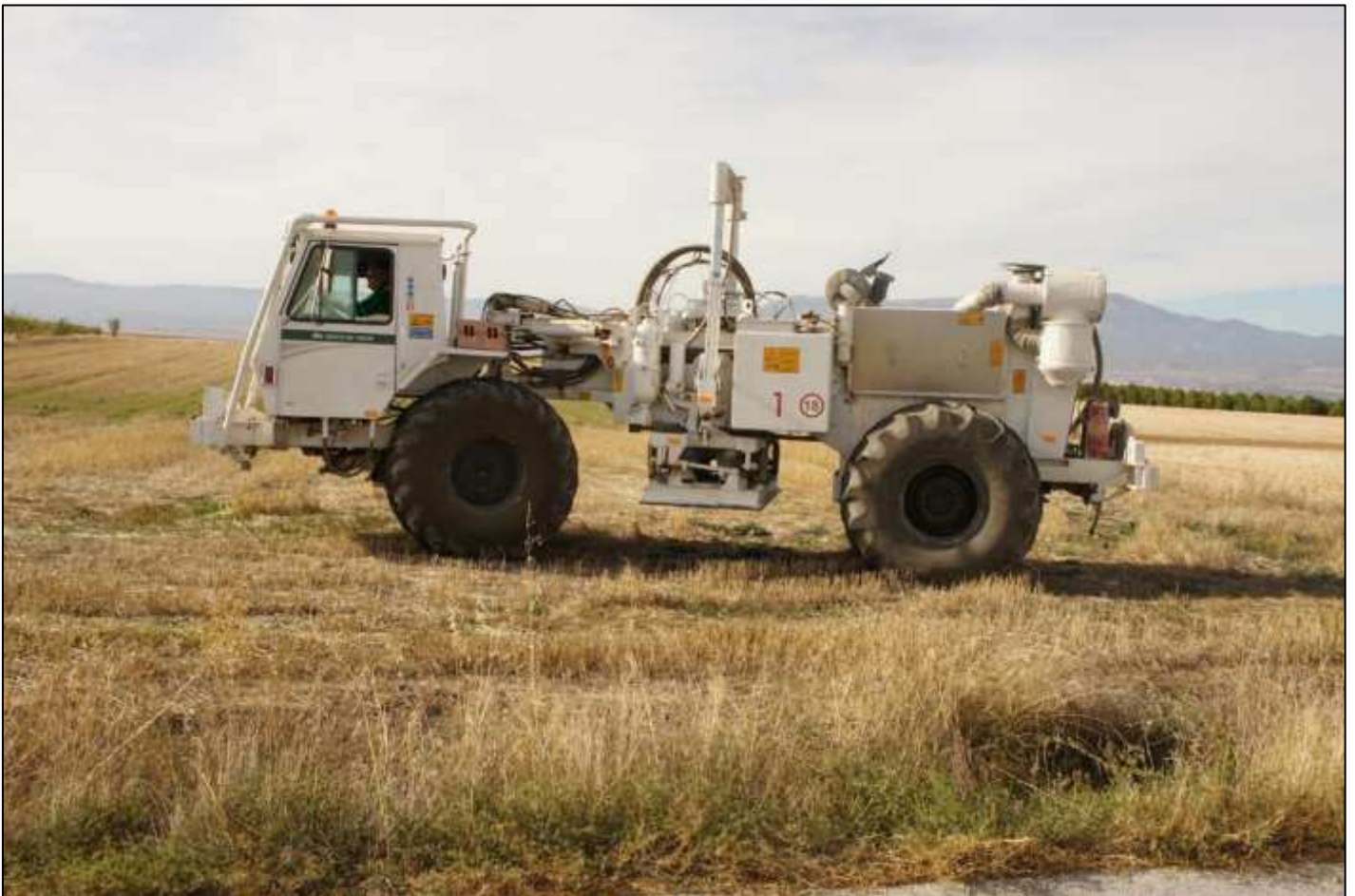
Plate 2.2: Vibroseis used as energy sources for onshore oil and gas exploration process (Source: REN, 2024).
