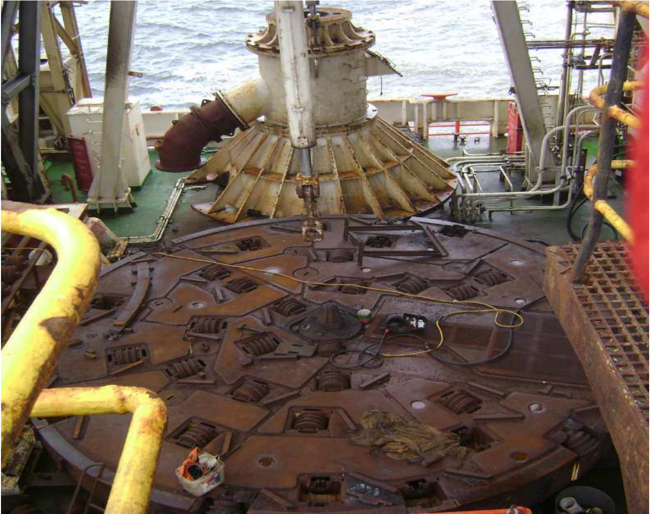
Plate 3.8: Overhead view of the cutting face of the Wirth Drill (note the individual wheel-cutters embedded in the circular disc (Source: DBMN, 2021).
