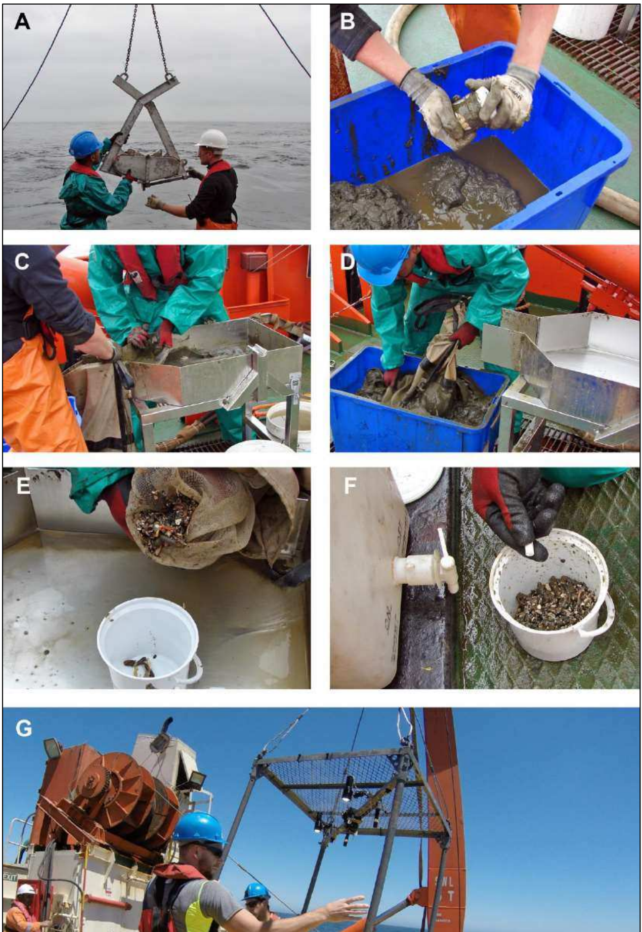
Plate 7.1: Sampling equipment used for collecting and processing samples during each DP Star grab sampling campaign: A – Van Veen Grab with impact trigger; B – collection of sediment; C – seamless transfer of sample from processing tray to 1 mm sieve bag; D – washing of sample through 1 mm sieve bag; E – washed macrofauna sample; F – addition of chalk and 10% formalin solution; G – drop-camera (Source: Biccard, et, al., 2024).
