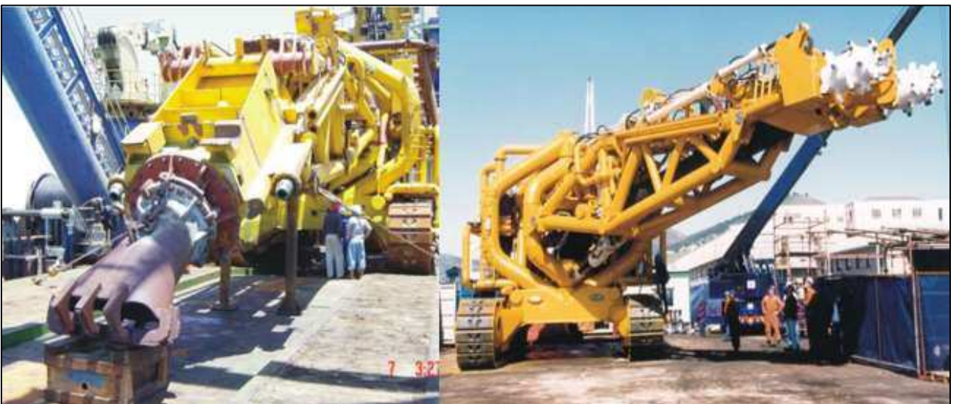
Plate 3.9: Typical seabed crawlers with different recovery head configurations (Source: DBMN, 2021).
