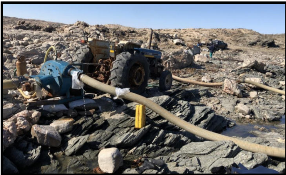
Figure 5: Picture showing a tractor, gravel pump, and suction hose (Source: Anonymous, n.d.).
