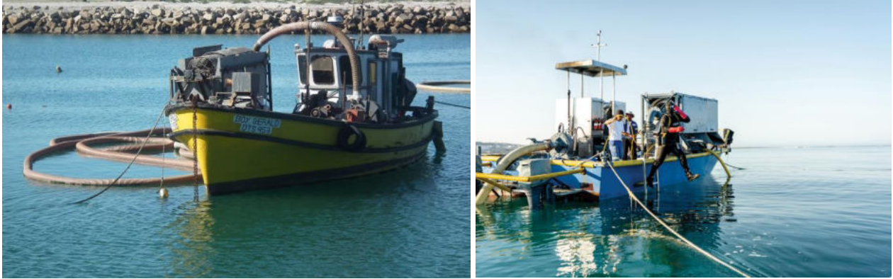
Figure 4: Pictures showing the boats typically used for shallow water mining operations (Source: Mr Hans Hückstedt, Chief Geologist, Namibian Diamond Company (Pty) Ltd).
