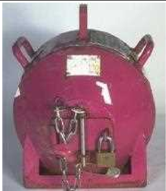
Photo 5-9 An example of a pig containing a Am-241Be SRS
