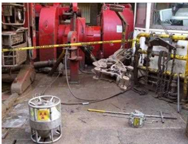
Figure 2.1 Photograph of an oil platform showing typical well-logging transport containers and source transfer tools 1 .
