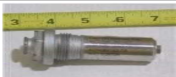
Photo 5-7 An example of a sealed source containing Am-241/Be
