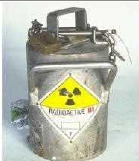
Photo 5-8 An example of a pig containing a Cs-137 SRS
