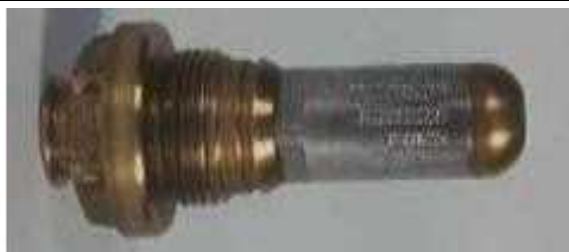
Photo 5-6 An example of a sealed source containing Cs-137
