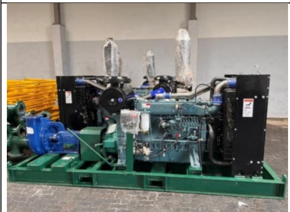
Photo 4-8 Diesel driven centrifugal pump
