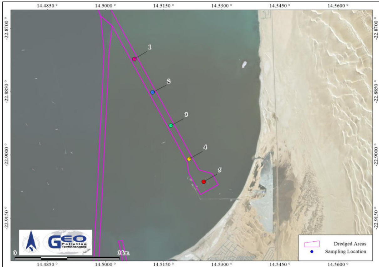
Figure 9-14 Sediment sampling locations prior to capital dredging of the North Port entrance channel (Botha, 2015)
