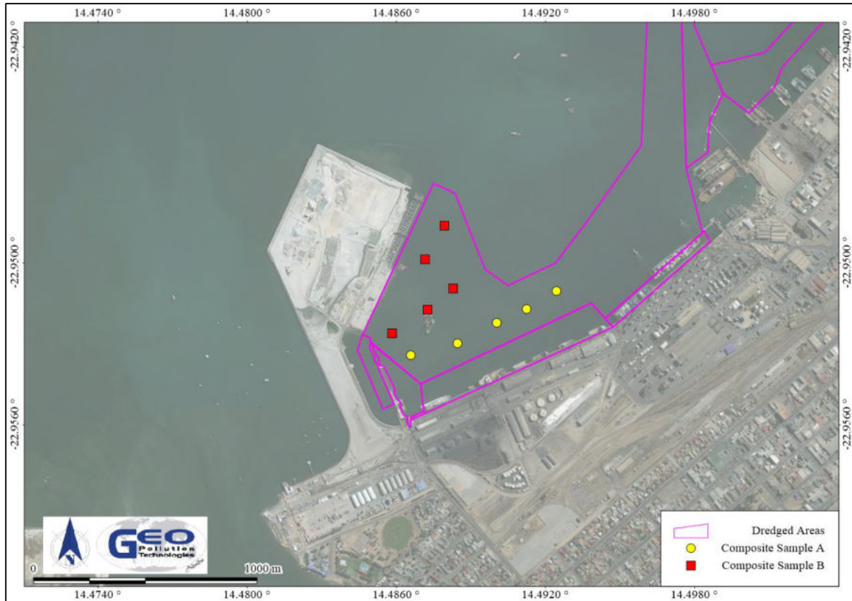
Figure 9-12 Sediment sampling locations prior to dredging at the new container terminal (Botha, 2014)
