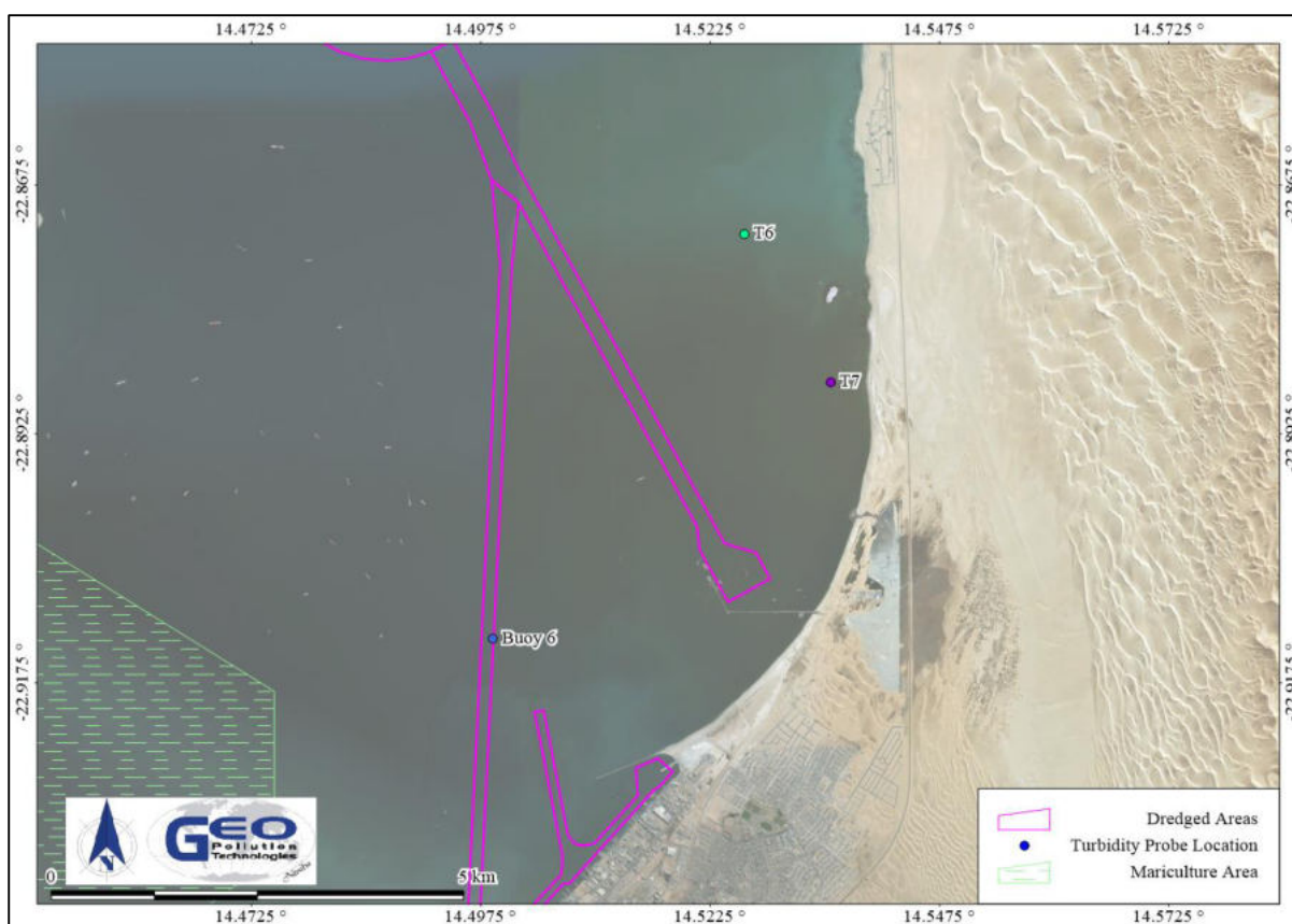
Figure 9-17 Locations for determining baseline turbidity and total suspended solids conditions prior to the dredging at the new fuel terminal (Botha et al., 2015)
