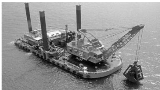
Photo 6-1 Typical grab dredger (from Vlasblom, 2003)
