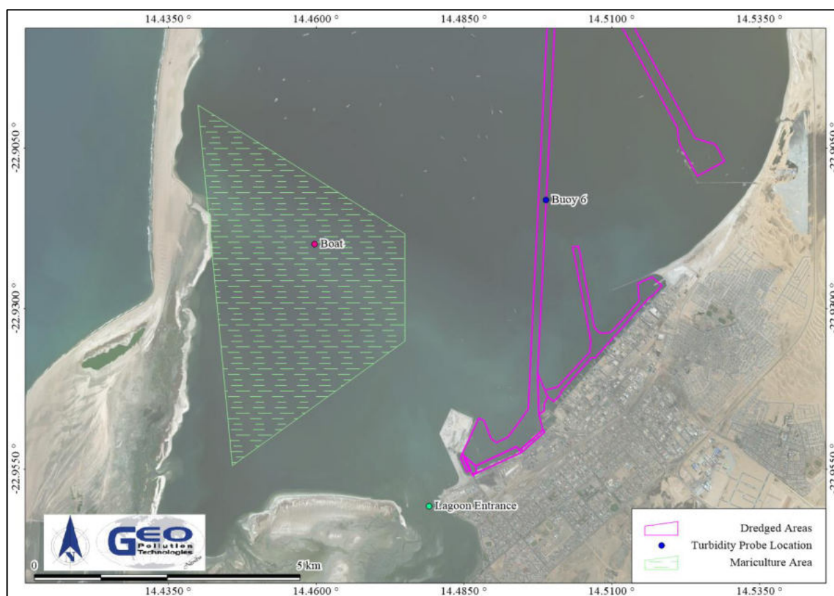
Figure 9-16 Locations for determining baseline turbidity conditions prior to the dredging at the new container terminal (Botha et al., 2014)
