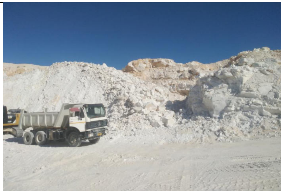
Dolomite rocks transported to processing plant using tipper trucks
