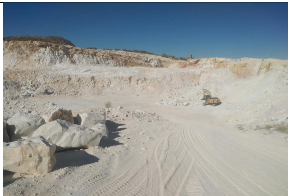
Mining pit (Open Cast) where dolomite rock is mined using excavators and loaded on tipper trucks
