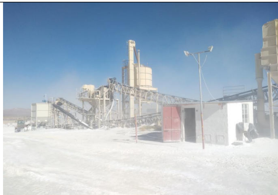
Processing plant where dolomite rock is crushed and processed into dolomite ore
